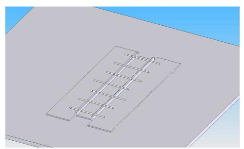
Step 7: Cut overlength rungs from 0.010: styrene rod, place them in the half-holes and bond with styrene solvent. Be careful not to get any between the stiles and the fixture.
