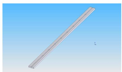
Step 4: Drill #80 holes in rung locations. (Now you see the reason for the bevels.) You might want to make a fixture for this using stile halves that are glued along their full lengths. Drill rung holes in that, glue lengths of styrene to a styrene plate spaced so as to hold the drilled double stile securely in place, then drill through the rung holes all the way through the styrene plate. Now you only have to put stile material between the spacers and drill them from the plate side.
