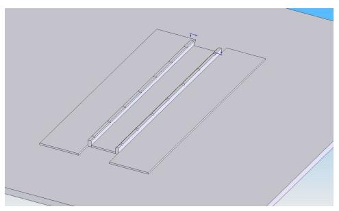
Step 6: Cut the stile halves to length and place in fixture.
