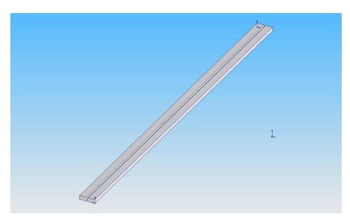
Step 3: Cut the length of stile material in half, glue the two halves together AT THE ENDS ONLY with the beveled edges facing.
