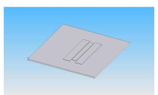
Step 5: Make a rung mounting fixture to hold the stiles upright. Size the center spacer for the desired ladder width.
