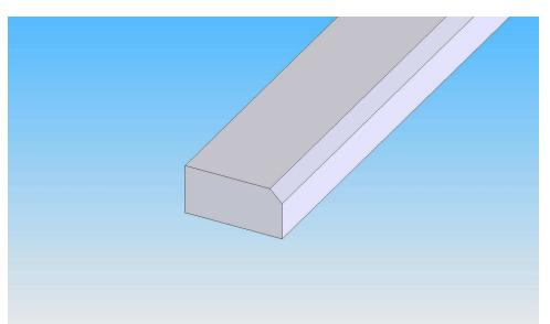
Step 2: Draw a blade along a long edge of the stile material to "break" it slightly. Shown exaggerated here.)
