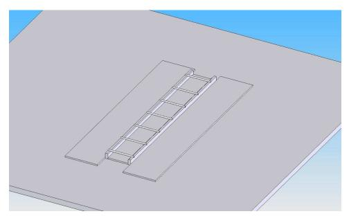
Step 8: Cut rungs to length. A single edge razor blade works well for his.
